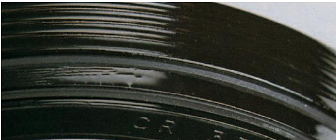
**Damaged O.D. beads**
