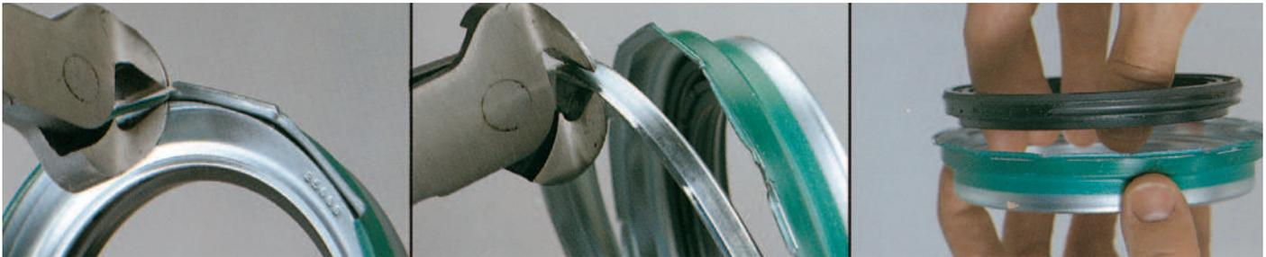
Use pliers or end cutters and work your way all the way around the seal, straightening the outer cup flange.
