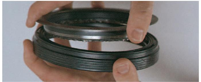
Pull the two components apart. Then set the sleeve assembly aside (the top component shown above). Place it carefully where it is out of the way, but won't be disturbed.
