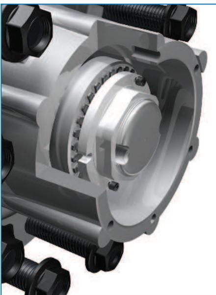
This system is intuitively easy to install and service, and requires no special tools. The spindle locking nut is now available in steering, drive and trailer sizes.
