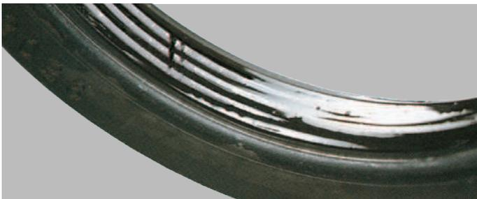
**Damaged I.D. beads**
