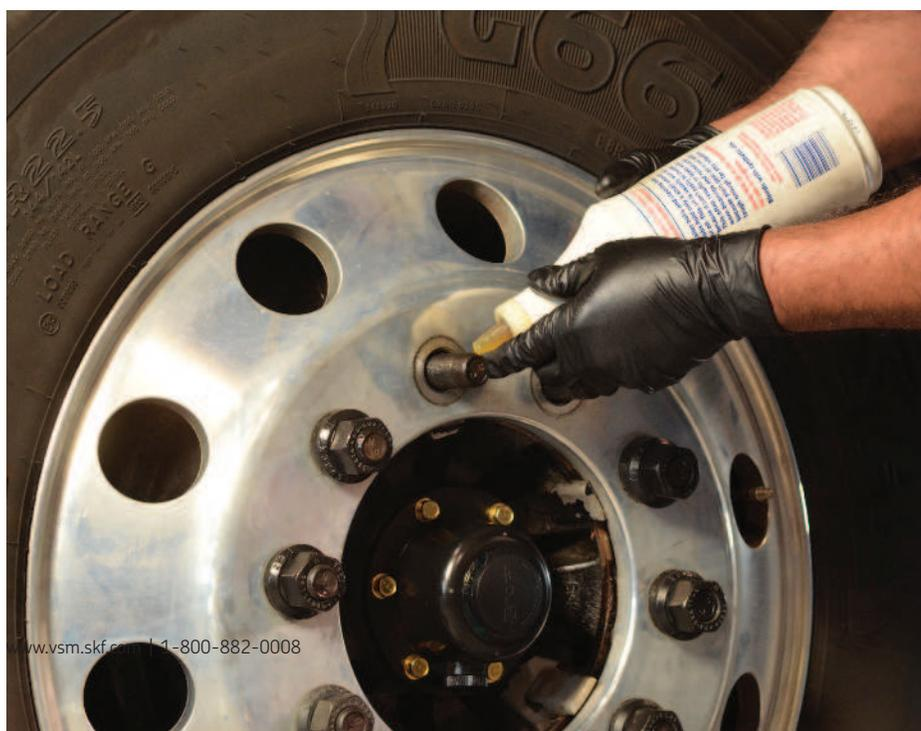
SKF recommends placing a small bead of oil on the end of each stud before installing the two-piece wheel nut
