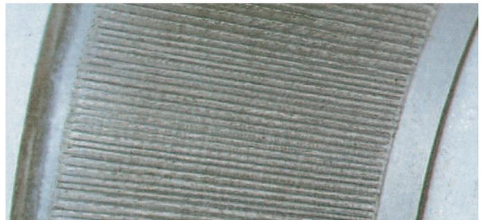
*Light pitting can be caused by electrical arcing. The probable cause is electrical welding grounded through the shaft.*
